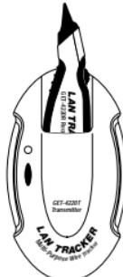
To access the adapters, open the back of the transmitter. All five plugs are contained in individual slots. During use, the appropriate plug can be pulled out of the slot, and the cover closed. The On/Off button is located on the front of the housing. To activate the unit, press this button once. The LED will blink, indicating that a signal is being transmitted. The unit can be turned off by pressing this button again. To conserve battery life, the unit will turn itself off after 30 minutes.
